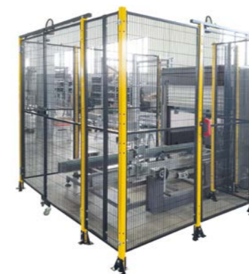
Fig. 11 Perimetral safety protections CAR
